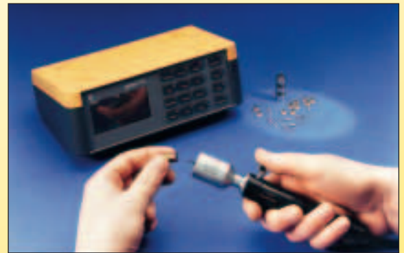
D100 Digital display using small bore 1.15-1.30mm 2 point measuring head.
